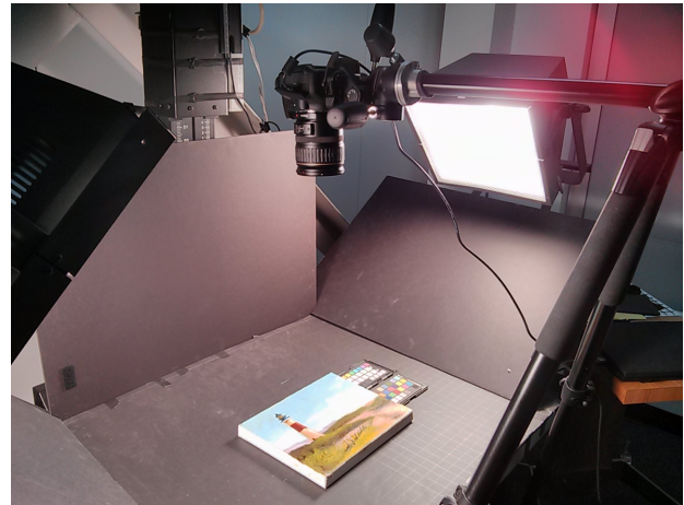
Figure 2. Painting acquisition. Canon 60D is mounted perpendicular to the painting on the stage. Two diffuse studio lightings are put on both sides at 45° from the stage. ColorChecker is used to correct image white balance after capturing.
