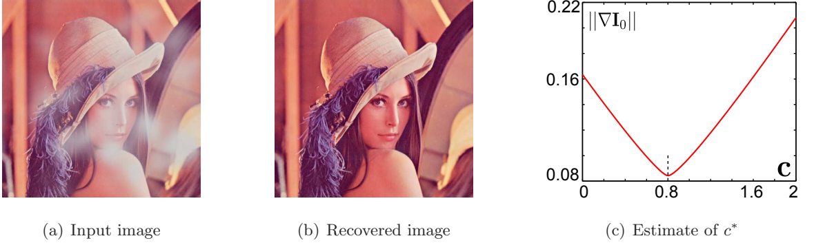
Figure 5.4: Simulation results for estimating the aggregate of outside illumination c based on Equation (5.10). (a) A synthetic image with a dirty-lens artifact is generated using the lens dirt pattern extracted from Figure 5.3(c). (b) Equation (5.10) is used to recover an artifact-free image, with a mean absolute percentage error of 0.44% compared to ground truth. (c) A plot of \|\nabla I_0(x)\|_1 versus c . The optimal estimate, c^* , has a 0.25% error compared to the ground truth.
