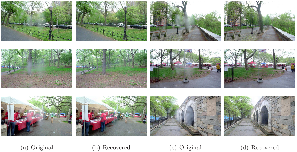
Figure 5.8: Removal of the dirty-lens image artifacts from a video without calibration. Based on the estimated attenuation map and the scattering map, dirty-lens artifacts can be removed for each frame. We show several examples where (a) and (c) are the original frames, and (b) and (d) are the recovered images.
