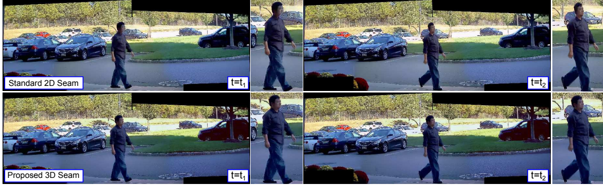
Figure 6. Composition results for stitching three aligned videos. Top: we use the standard seam finding and blending method in AutoStitch in OpenCV, which is based on 2D graphcut. Bottom: we use the proposed spatial-temporal seam finding method, which is a 3D weighted graphcut method. The alignment is the same for both methods. Each row shows two stitched frames, with zoomed insets. As shown, the standard 2D seam method has artifacts and temporal inconsistency while the proposed 3D seam method works well.
