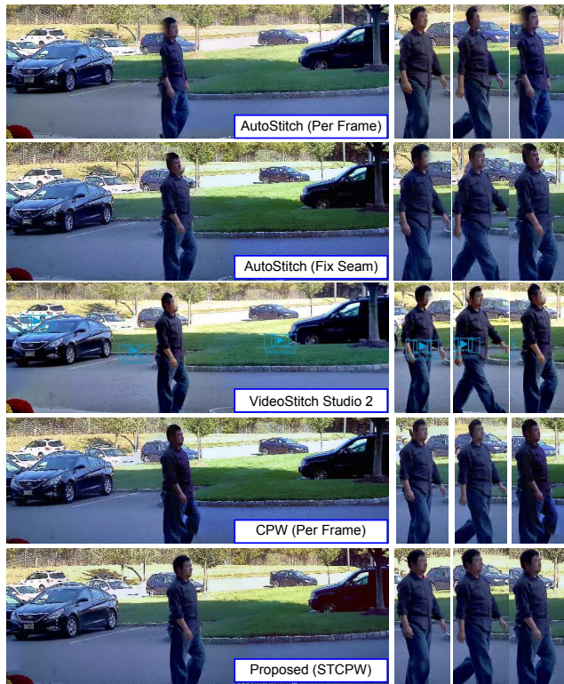
Figure 1. Video stitching is non-trivial. This figure shows the stitching of three video cameras, with AutoStitch from OpenCV (each frame stitched separately or using a single common alignment for all frames), a commercial software VideoStitchStudio2 [1], parallax-tolerant stitching ( i.e. , CPW) for each frame separately [20], and our proposed method ( i.e. , spatial-temporal content preserving warping STCPW). Left : one of the stitched frames. Right : zoomed insets over multiple frames. Please refer to the supplementary material for stitched videos.
