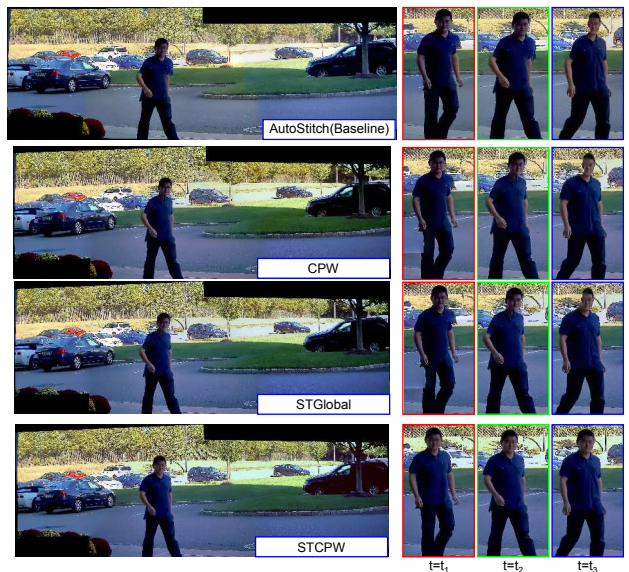
Figure 7. Video stitching results of three PointGrey Cricket cameras. Left: one of the stitched frames. Right: zoomed insets over multiple frames. Note the distortion and cut-through artifacts on the foreground moving object. Please refer to the supplementary material for stitched videos.
