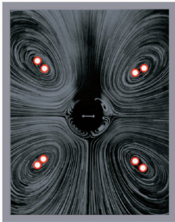
Fig. 11. Detecting vortexes and saddles in the fluid image using the proposed algorithm.
